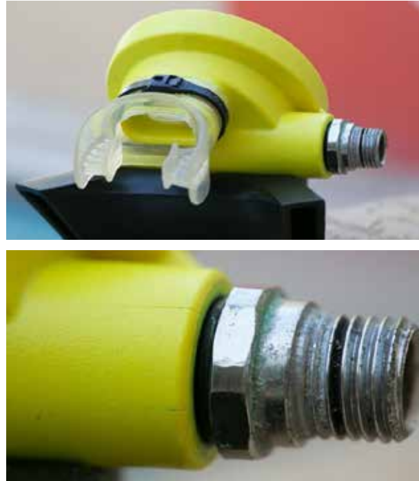
Figure 3-5. Plastic second-stage regulators with microfractures
